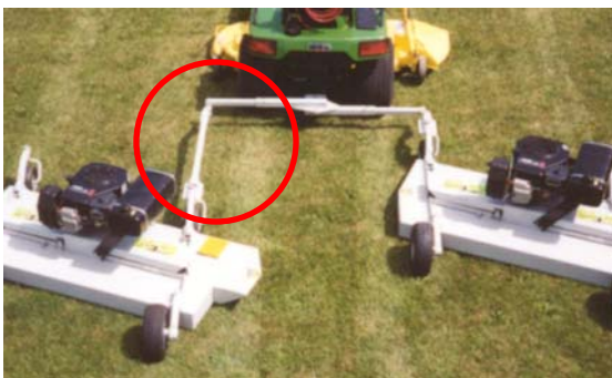
Long Tongue Extension Part # 900008 Left and right wing mower set-up.
